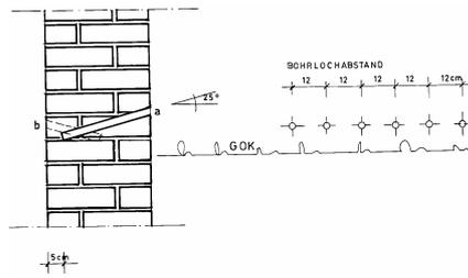
Fill hollow masonry, e.g. double leaf cavity masonry with a loose core filling, narrow cracks, etc., with Remmers Injection Mortar first.
